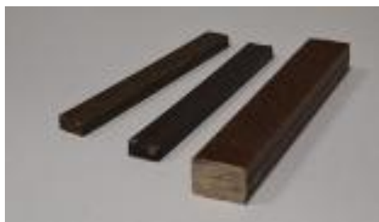
Figure 8. A new wood-plastic composite based on recycled polypropylene, alkaline-treated pine sawdust, containing suberinic acids as an internal lubricant
